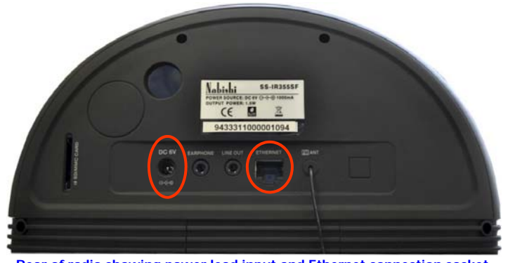
Rear of radio showing power lead input and Ethernet connection socket
