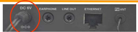
Plug in the supplied power socket at the rear of the internet radio
